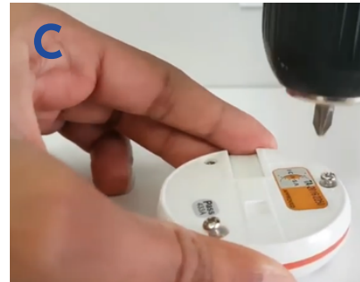
C. Remove the 3 screws to replace the battery.
